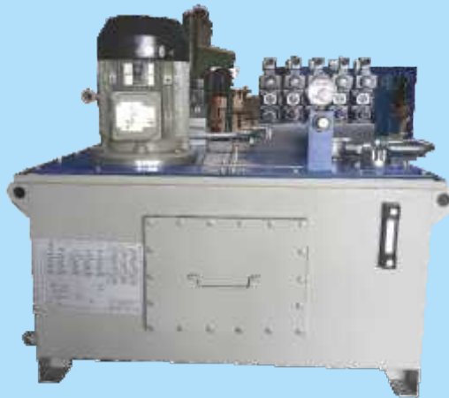
GDC Machine Operating Power Pack
